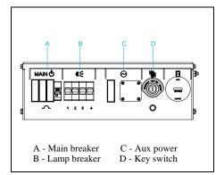
Figure 3.8 Circuit breakers/power switch
